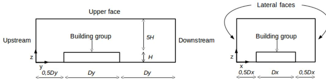
Figure 3. Dimensions and boundary conditions of the considered domain.
