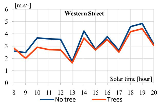
Figure 9. Wind speed on the last day of simulation.
