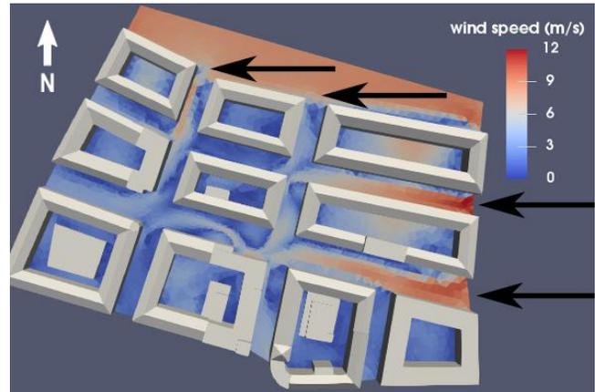
Figure 8. Wind distribution without tree at 15h. Wind original direction is from East.
