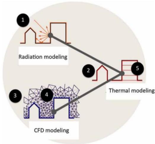
**Figure 1.** The coupled modules in SOLENE-microclimat [13].
